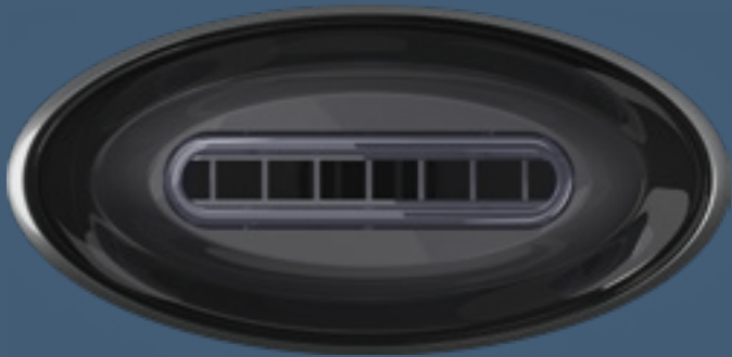
Jacuzzi® PowerPro® PX swim jet The wide-stream PX swim jets channel a high volume of water into a concentrated flow with an air-free stream that forms the optimal swim lane. Vertical blades evenly distribute water for a predictable swim.
